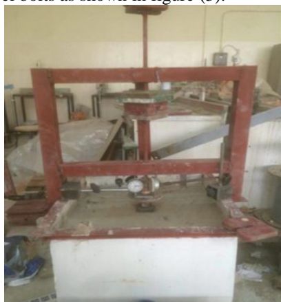
Figure (3). Large box with the frame loading
