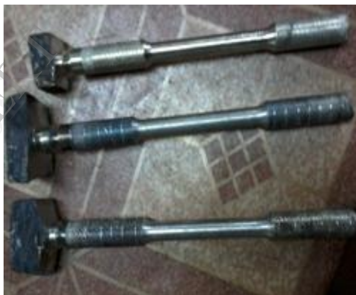
Fig 1. Testbars used for mechanical testing
