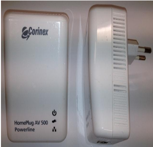
Fig. 11 PLC modems Corinex AV500 Powerline
