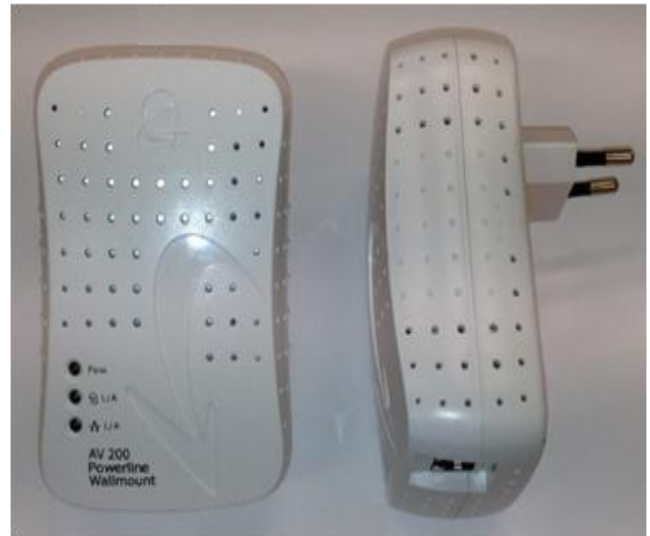
Fig. 5 PLC modems of the brand Corinex AV200 Powerline Ethernet Wall Mount
