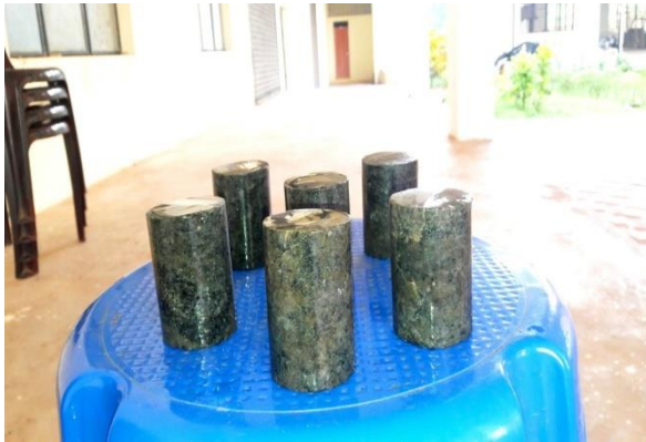
Fig. 2. Rock samples for Point load Index test
