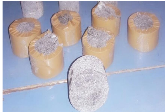
Fig. 1. Rock samples for Brazilian test
