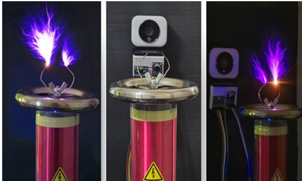
Figure 2. Experimental setup showing the Tesla coil plasma discharge used as the physical entropy source during data collection. A camera, microphone, and accelerometer observe visual, acoustic, and mechanical variations of the plasma and transmit the captured data to the processing system.
