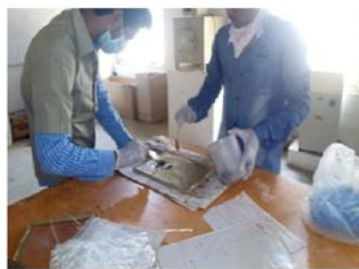
Fig.2 Applying Epoxy for second layer
