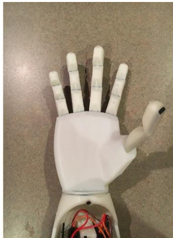
Figure 2.2: 3D printed prosthetic arm [13]
