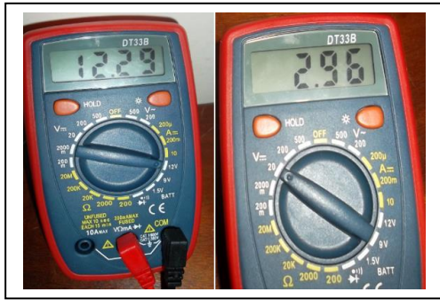
Fig. 5. Measured battery and input voltage to the microcontroller unit (MCU).
