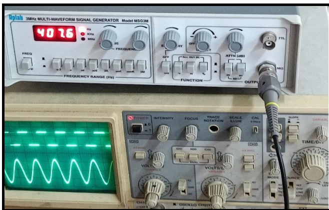
Fig 5: 400 Hz square wave and its filtered output
