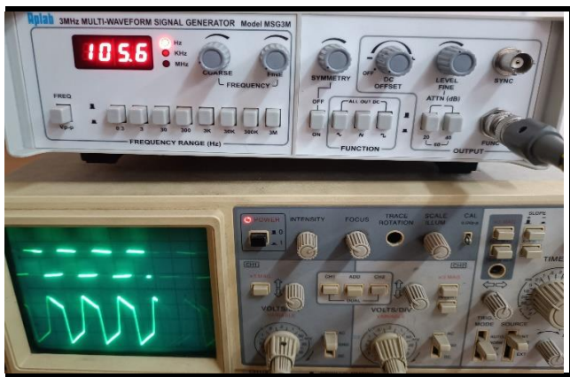
Fig 4: 100 Hz square wave and its filtered output
