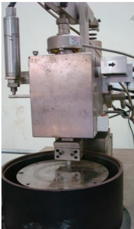
Fig 1: Pin-on-disk wear test equipment
