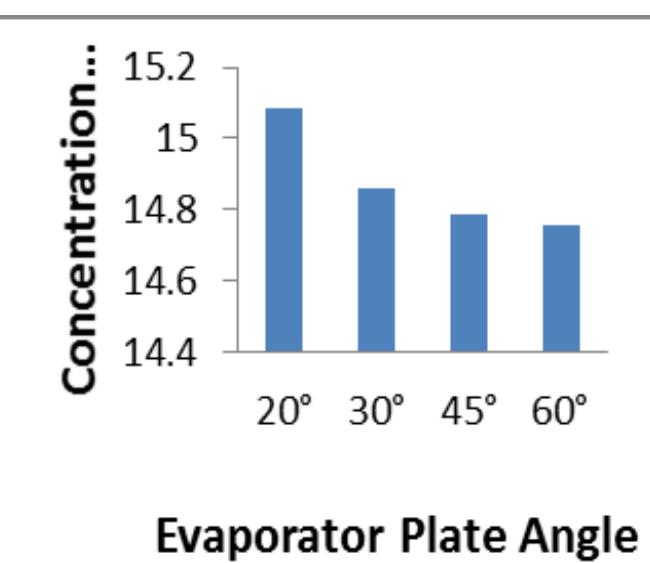
From the above fig it can be seen that as evaporator plate angle increases the concentration rate decreases.
