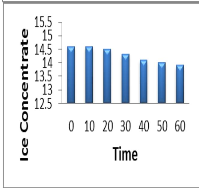
At 60 degree plate angle an orange juice of 0.5 liters quantity can be successfully concentrated from 14.6 to 15 Brix in batch process.
