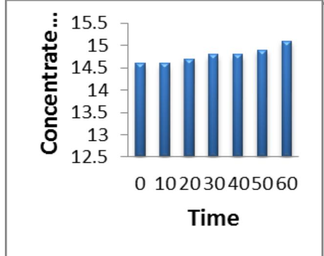
At 30 degree plate angle an orange juice of 0.5 liters' quantity can be successfully concentrated from 14.6 to 15.2 Brix in batch process.
