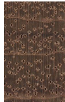
Fig. 8. Microscopic Structure of the Guibourtia Tessmannii : and-grain cutting [1].
