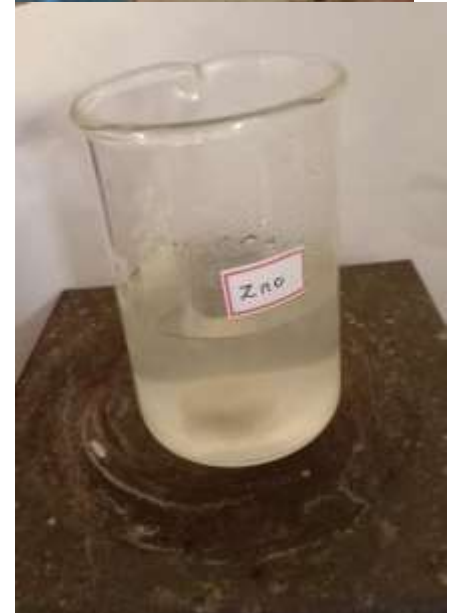
a) Boiling of aloe vera gel with Distilled water (50°-60°C)
