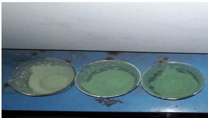
Fig 2 Synthesized powder of ZnO
