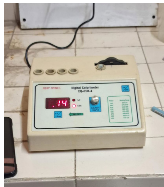
Figure 5.5: Colorimetry test to find %P
