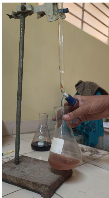
Figure 5.3: Titration with 0.1 mol HCl solution to find %N
