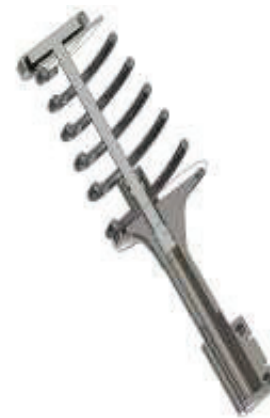
Fig. 8. SolidWorks CAD representation of the rear dual-link strut assembly.
