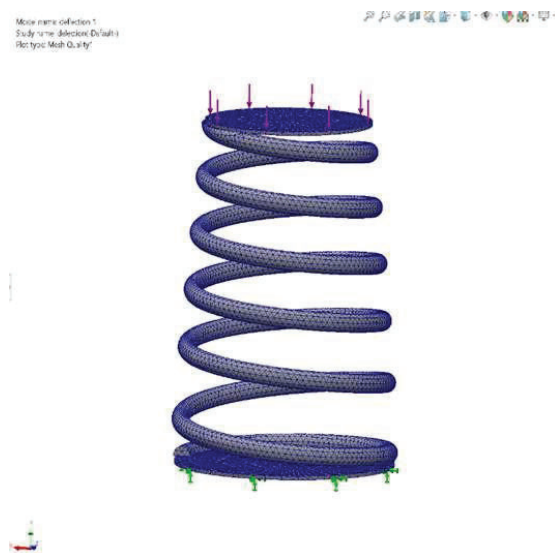
Fig. 9. Finite-element mesh applied to a suspension spring for static-compression analysis.
