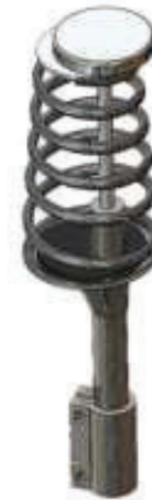
Fig. 7. SolidWorks CAD representation of the front MacPherson strut assembly.
