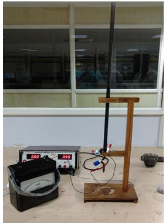
Fig. 1. Magneto-burette test setup
