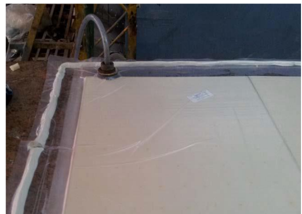
Fig 5. Sandwich composite fabrication by vacuum bagging process
