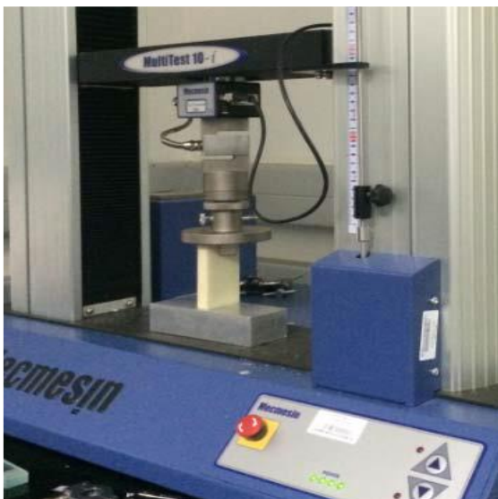
Figure 14. Edgewise compression testing
