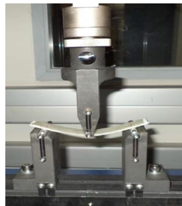
Figure 11. Flexural testing of laminate
