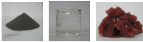
Fig. 1: Carbonyl Iron, Silicone Oil and Grease
