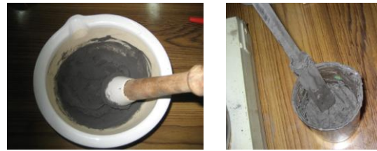
Fig. 2: Mixing process for preparing MRG
