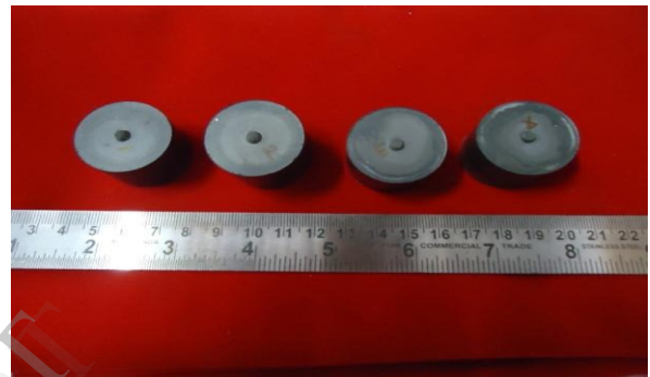
[Fig3] Ti6Al4V Green compacts
