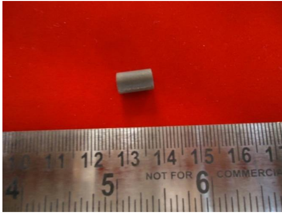
[Fig5] 10mmX10mm Compression Testing Specimen.
