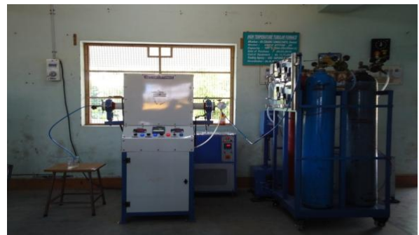
[Fig4] 1800c Capacity Tubular Sintering Furnace
