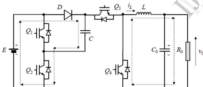
Fig.3. Current path in state 2 configurations
