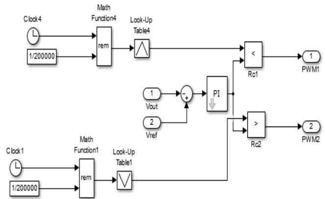
Fig. 5. Simulink PI-PWM gate signals for switches
