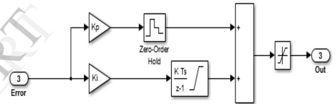
Fig. 6. Discrete PI Controller
