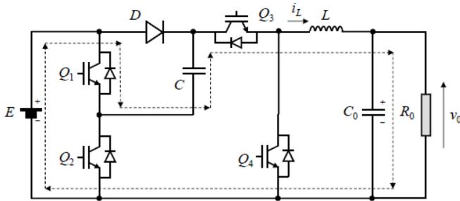
Fig.2. Current path in state 1 configuration
