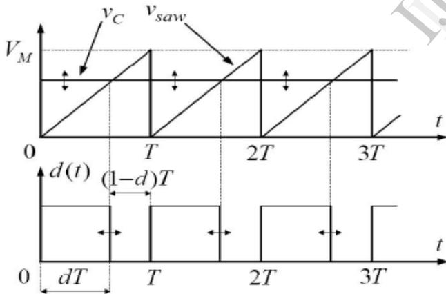
Fig. 4. Generation of the switches gate signals
