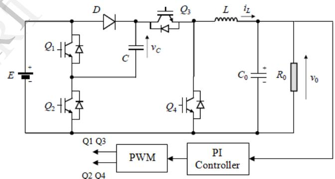
Fig. 1. Synchronous buck-boost topology with its voltage control circuit
