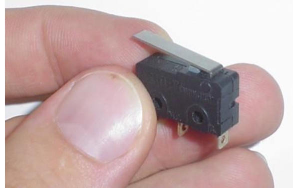
Fig. 3 Tactile Bump sensor
