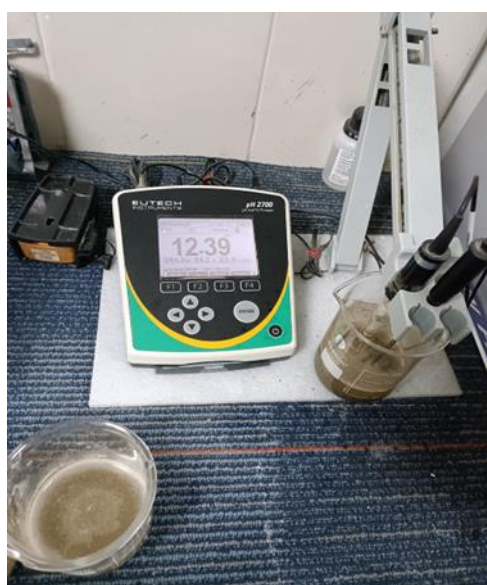
Fig. 2 pH Test Performed for Peat+Lime Mixing
