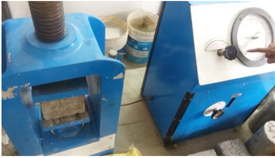
Fig 1-Testing of compressive strength of concrete
