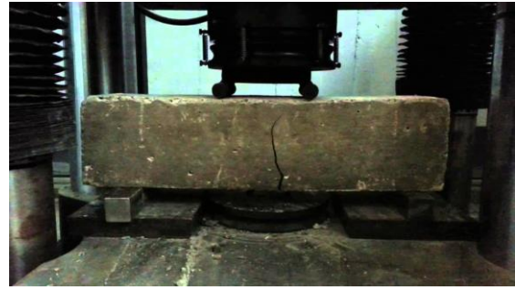
Fig 2:Setup of flexural strength of concrete
