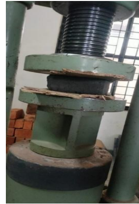
Fig 4: compressive strength testing on geopolymer concrete
