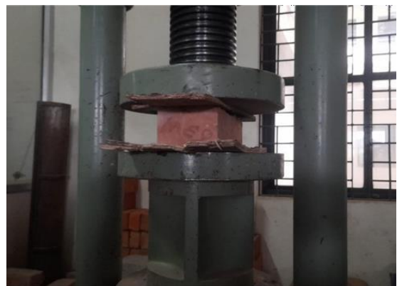
Fig 3: Compressive strength testing on brick
