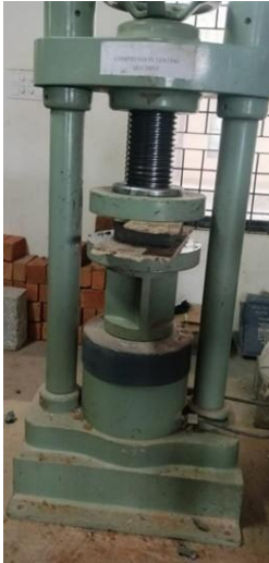
Fig5: Compressive strength testing on bamboo reinforced slab
