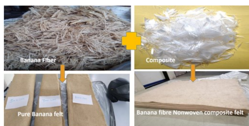
Fig. 3. The manufacturing process of nonwoven composite felt
