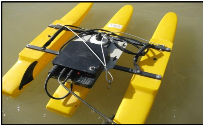
Fig. 3: SonTek River Surveyor ADCP
