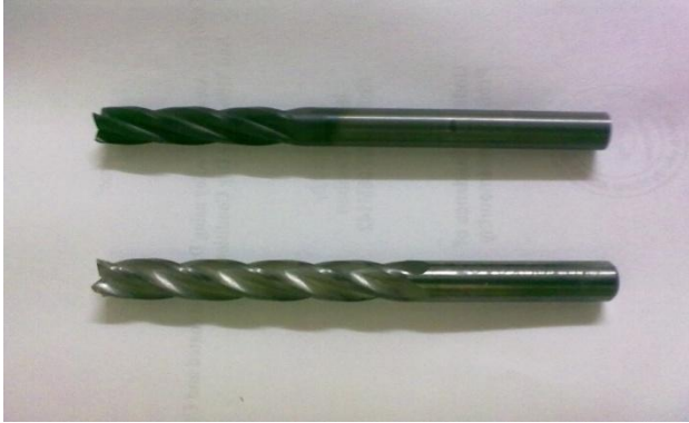
Fig.2 Diamond coated (top) and uncoated (bottom) Tungsten Carbide Tools
