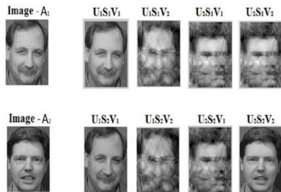
Result of swapping Two Orthogonal Matrices (U, V) Between Two High Resolution Images
