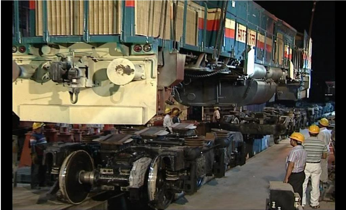
LOWERING OF 100 TONNE LOCO ON 2 BOGIES
