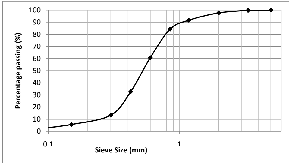
Figure 1: Particle Size Distribution curve for the sand used for the concrete production
