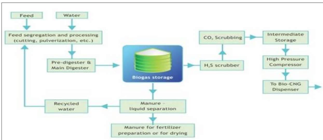
Figure 8: Process for production of biogas from press mud
