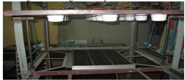
Fig 1.2: Developed sun simulator and module testing arrangement
