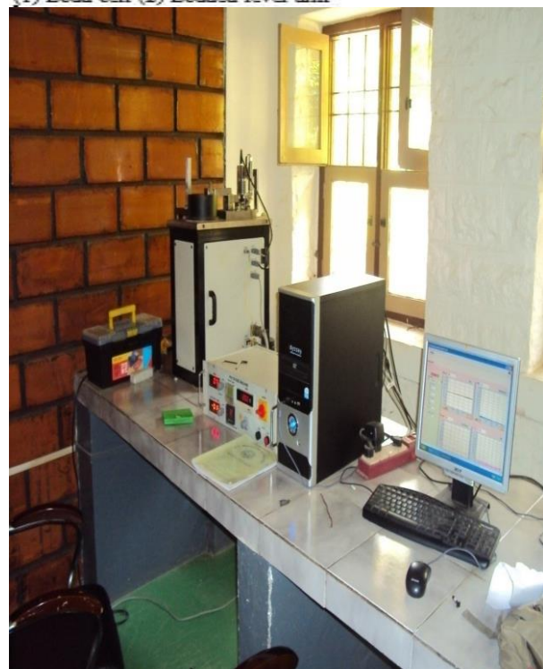
Fig 3.7: Experimental setup of pin-on-disc test apparatus
