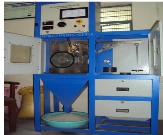
Fig 3.4: Picture of dry sand/rubber wheel abrasive wear test experimental setup
