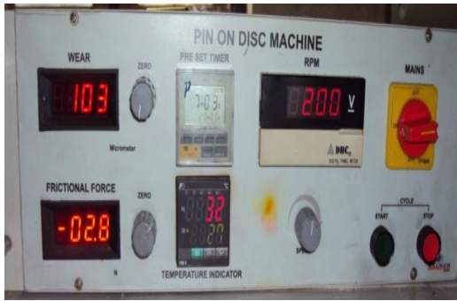
Fig 3.8: Control unit for computerized pin-on-disc test
