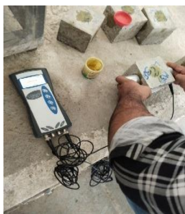
Fig 4. Cubes under UPV
