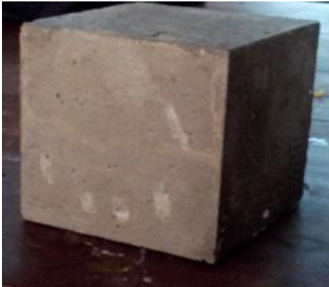
Fig 3 Cubes covered with water proofing compounds
