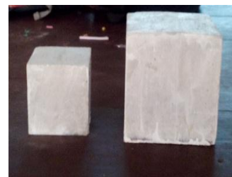
Fig 1 Cubes covered with acrylic resin based curing compounds
