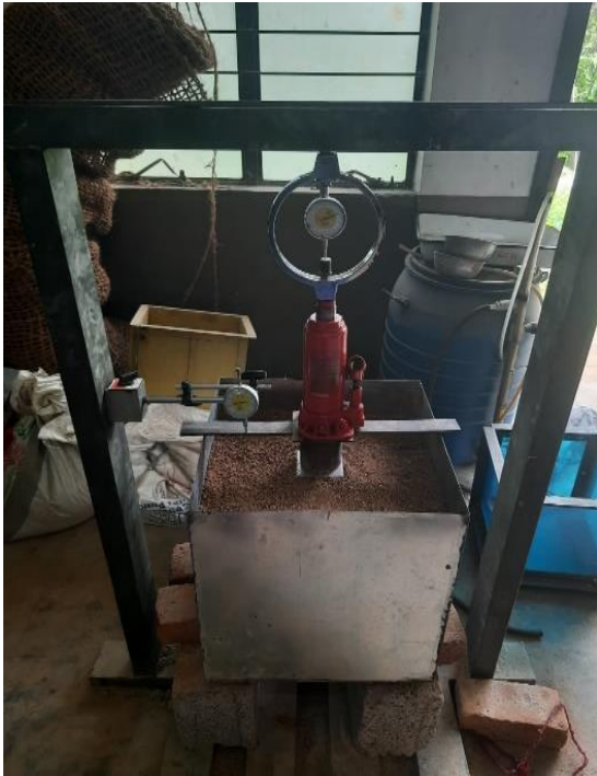
Fig 4.3 Plate Load Test
