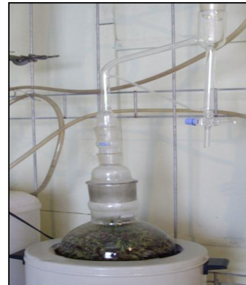
Fig.1 Patchouli plant, Oven drying and Oil extraction (Clevenger apparatus)
