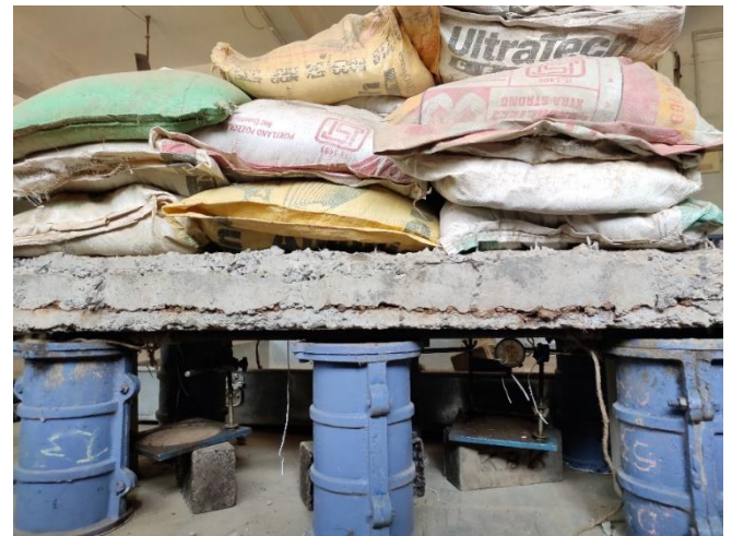
Fig.6 Loading & dial gauge arrangement
