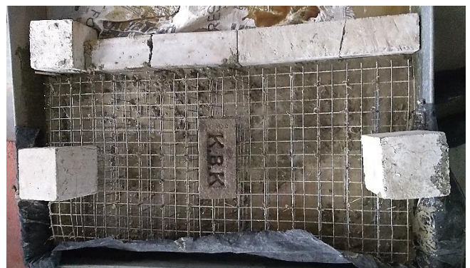
Fig.2 Laying of first layer of concrete
