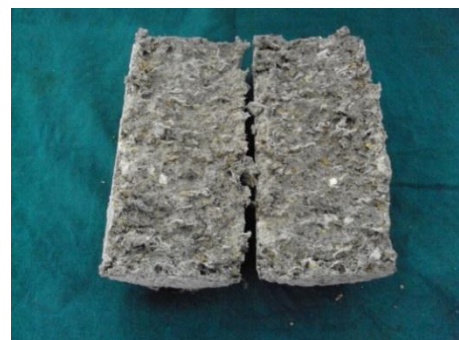
Fig 5: Split section of waste cloth concrete
