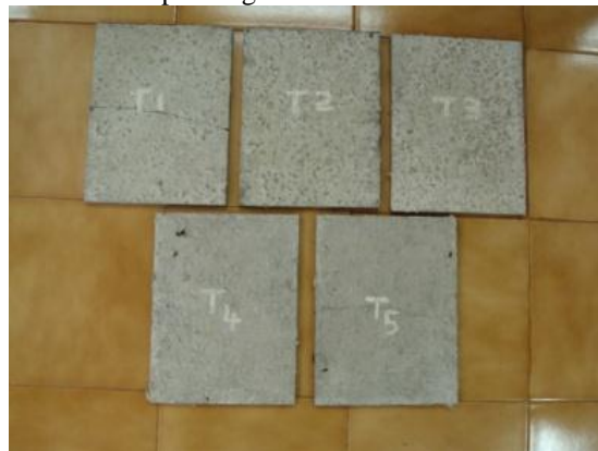
Fig 8: Tile specimens after impact test
