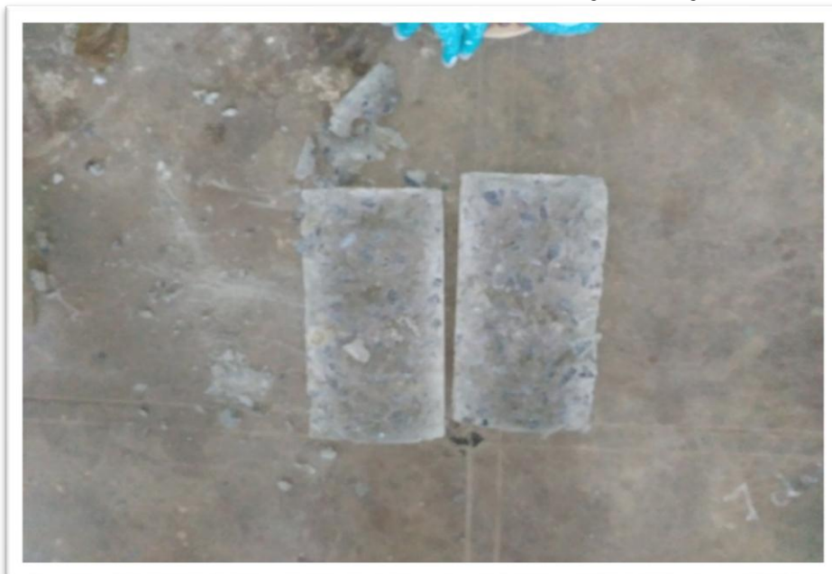
Fig 4 cylindrical specimen after failure
