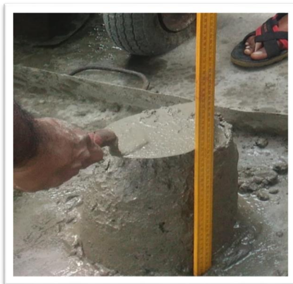
Fig 1 slump cone test of concrete
