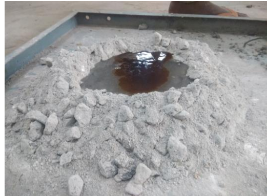
Figure 2: Dry mixture with alkaline solutions of NaOH, Na 2 SiO 3 and super plasticiser
