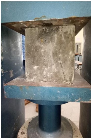
Figure 5:Testing of cube under CTM
