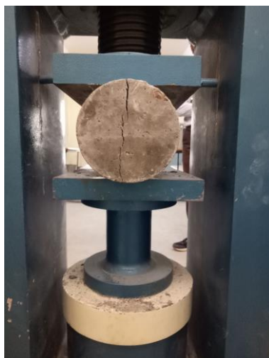
Figure 6:Testing of cylinder under CTM
