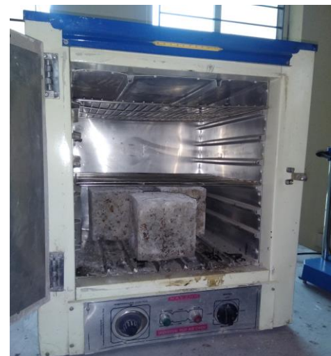
Figure 3: Oven dry for 12 hours at 60°C
