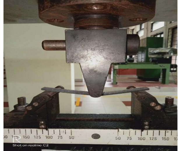
Fig. 4. Flexural test performed on UTM
