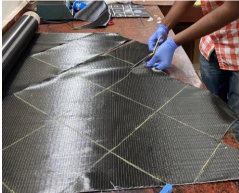
Fig. 2. Cutting of carbon fibre fabric into 45^\circ orientation
