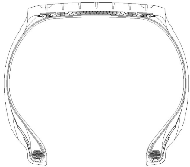
Fig.2. Two dimensional section model of walking wheel tire
