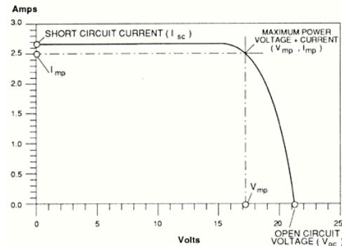
There is a point on the "knee" of the curve where the maximum power output is located. This point on example curve is where the voltage is 17 volts, and the current is 2.5 amps. Therefore, the maximum power in watts is 17 volts times 2.5 amps, equaling 42.5 watts. The power, expressed in watts, at the maximum power point is described as peak, maximum, or ideal, among other terms. Maximum power is generally denoted as "I (mp)."
