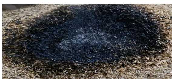
Fig 2: Rice Husk Ash (RHA) during the burning process
