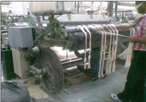
Figure 10. Dressing of warp yarns
