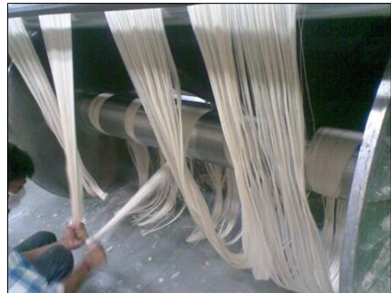
Figure 28. Damaged warp yarns are cut
