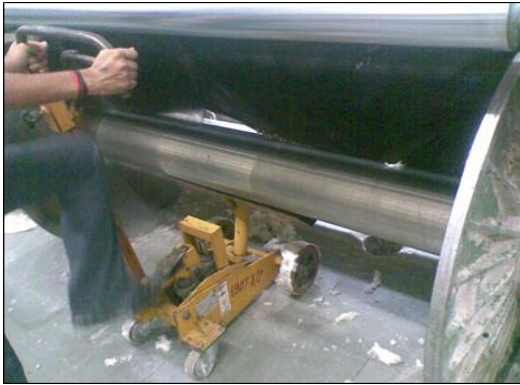
Figure 9. Unloading of empty beam
