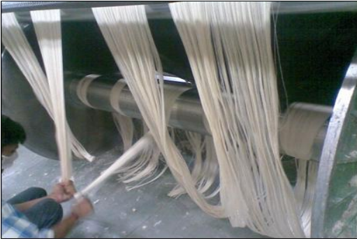
Figure 8. Cutting of warp sheet
