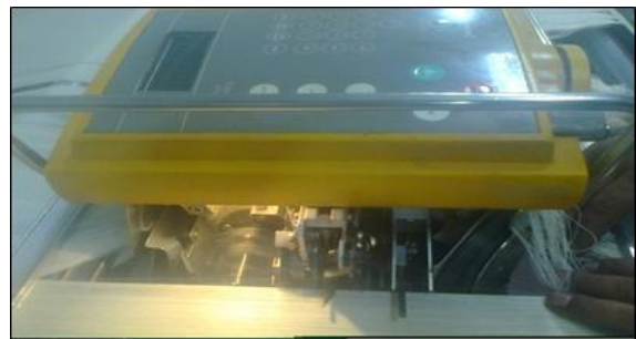
Figure 20. Knotting of warps yarns
