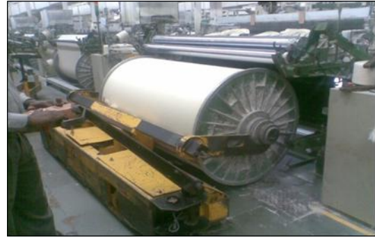
Figure 11. Loading of the new sized beam
