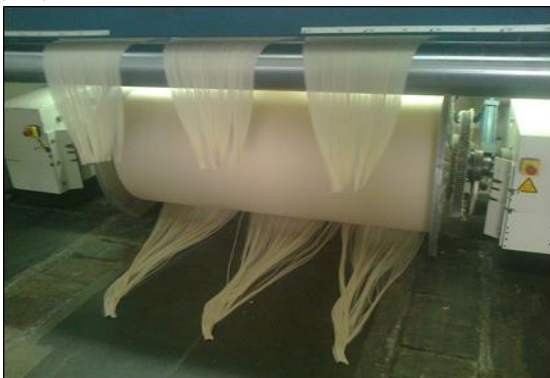
Figure 24. Unloading of the sized warp beam from sizing machine
