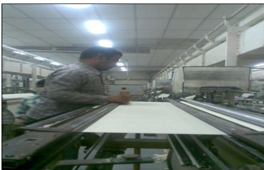
Figure 16. Warp sheet is clamped
