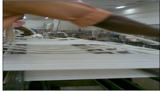
Figure 17. Dressing of loom warp sheet
