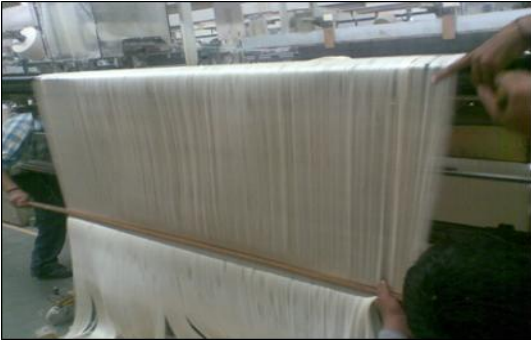
Figure 14. Damaged warp yarns is dragged out
