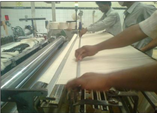
Figure 15. Dressing of new warp yarns
