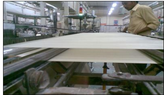
Figure 18. Clamping of loom warp sheet
