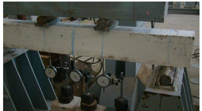
Fig 5: Testing of Beam Specimen
