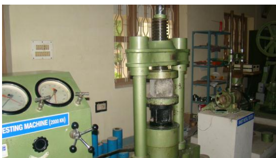
Fig 4: Compression testing of cube
