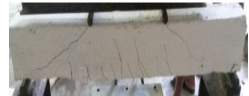
Fig.7 Typical crack pattern of shear beam specimen
