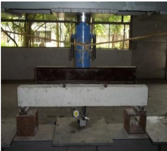
Fig. 3: Test setup for RC beam
