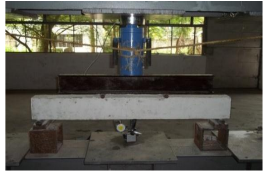
Fig. 3: Test setup for RC beam
